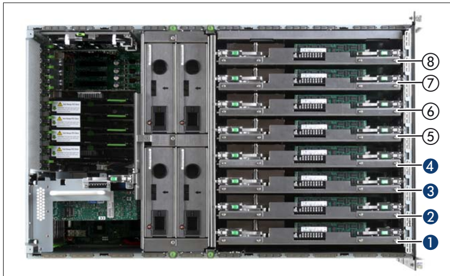
Figure 245: CPUMEMR numbering scheme
